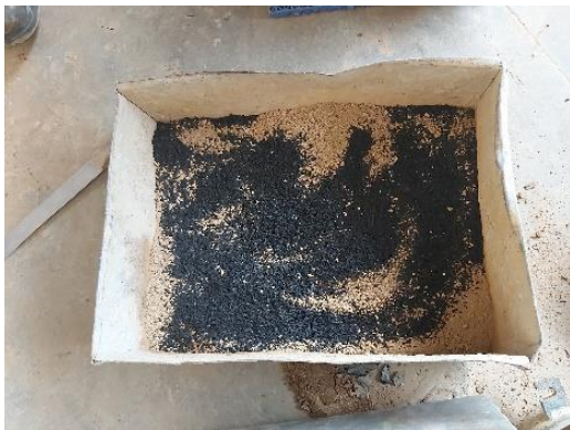
Fig.6 Soil-tyre crumb mix
